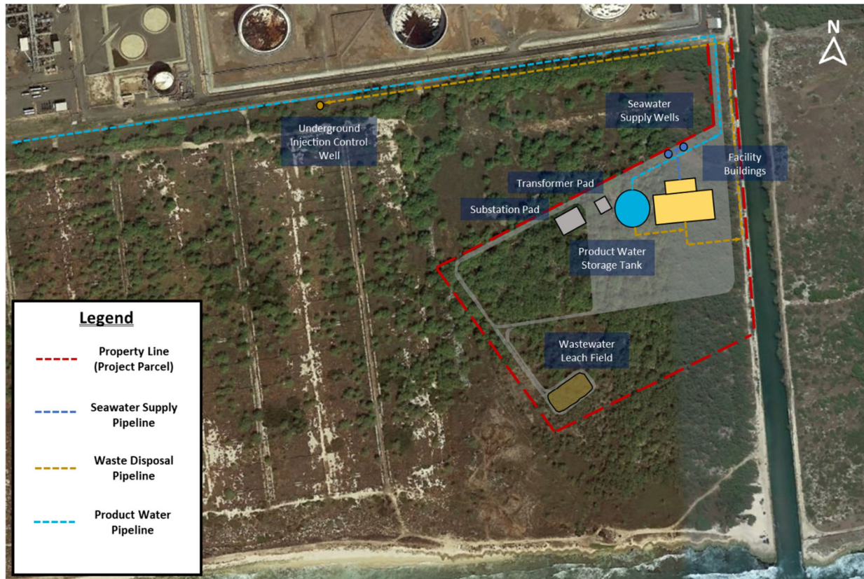
Figure 5. Kalaeloa desalination facility site layout
